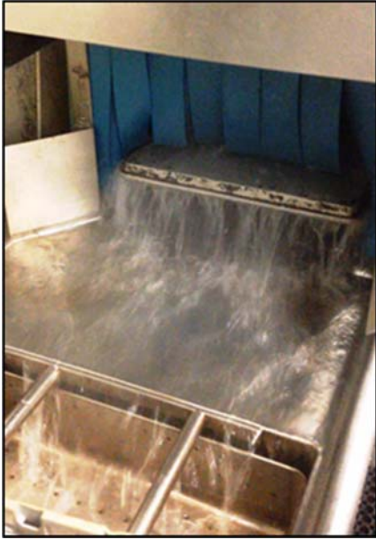
Figure 5. Overspray on soil side of conveyor due to washing sheet pans placed horizontally on the rack.
